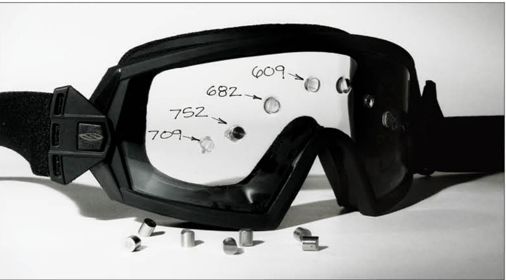
IMPACTED BY A 0.22 CALIBER, 17 GRAIN, T37 SHAPED PROJECTILE.
